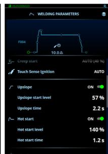
Intuitive view to adjust the parameters on welding channels.
