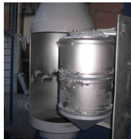
An upside down mounted bullet magnet for plastic granulate
